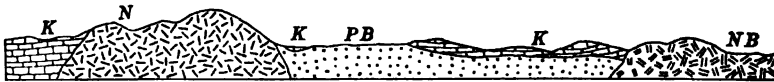
FIG. 185.—Section in the Uvalde quadrangle, Texas. (After Uvalde Folio, No. 64, U. S. G. S., 1900.) K , Cretaceous limestone and clay; PB , intrusive plagioclase basalt; N , intrusive nephelite-melilite basalt; NB , nephelite basalt. Illustrating syngeneses of ordinary basalt and "alkaline basalts." Horizontal scale, 1:95,000; vertical scale, 1:12,000.
